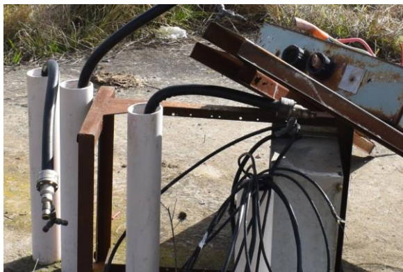
Figure 57: South Creek 4 – Detail of compressed air hoses and cut electrical connections at base of fuse box (or similar piece of equipment)
