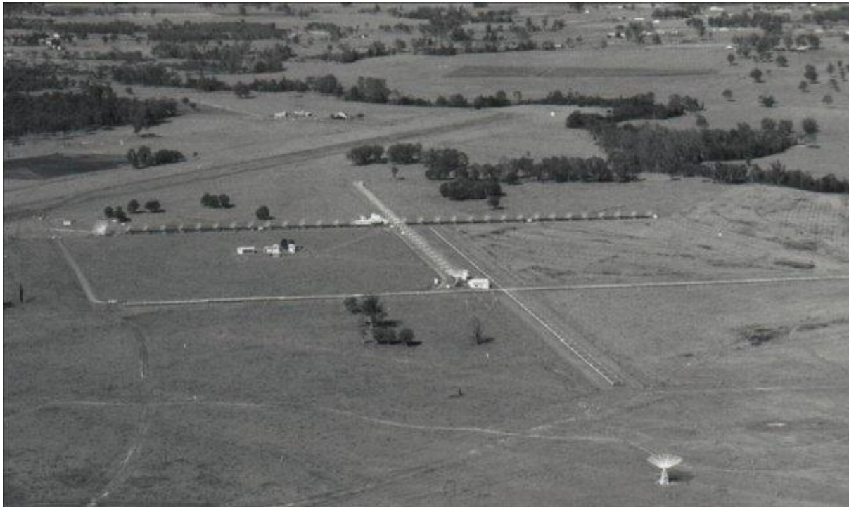
Figure 18: Undated view of the Chris Cross and Mills Cross from the north, showing three 13.7 m antennas, in the foreground and at the northern and eastern ends of the Chris Cross. The disused WWII air strip is visible in the background 57
