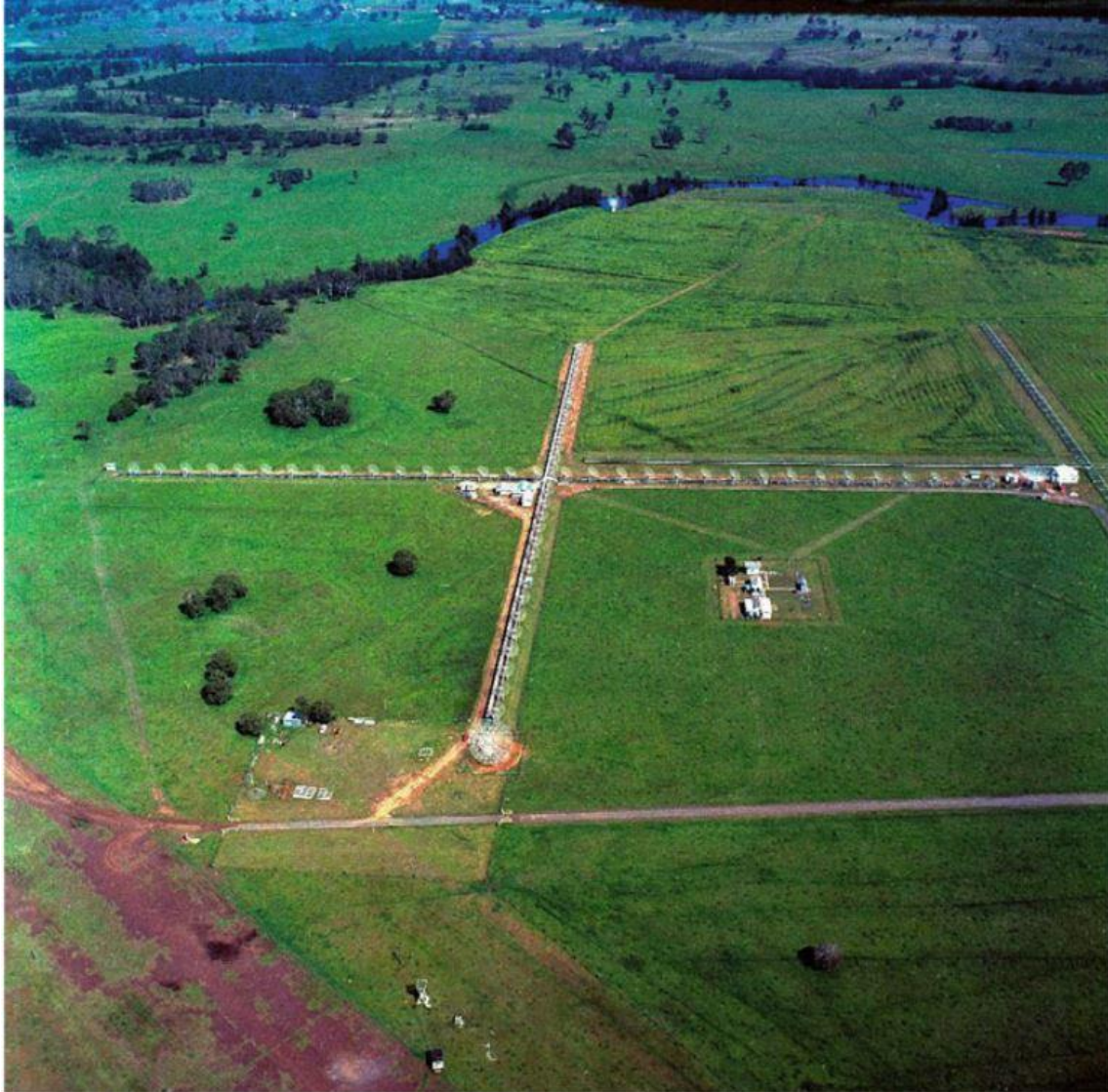
Figure 19: 1969 photograph showing the FST Site from the east looking west, showing two 13.7 m antennas at the northern (right) and eastern (front) end of the Chris Cross, and another one further to the west (background). The study area is still undeveloped 58
